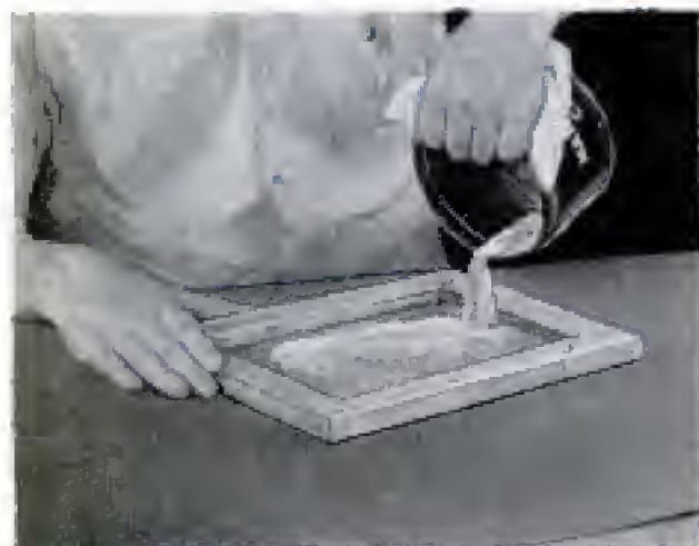
Above, melted beeswax is poured on glass of picture frame to a thickness of \frac{1}{8} in. Use only beeswax.
